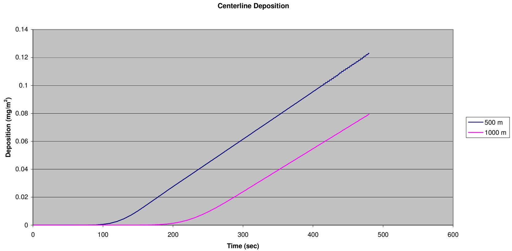
**Figure 1. Deposition as a function of time for non-evaporating case.**
