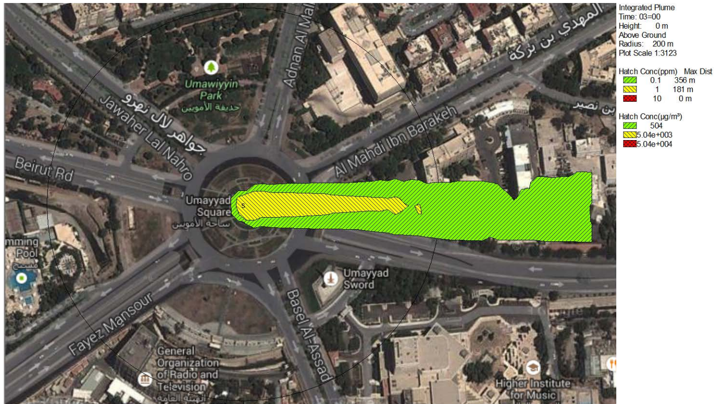
Figure 1 Plan view of all areas impacted by plume from Sarin release. Flat edge to the right is due to the plume exiting the calculation grid.
