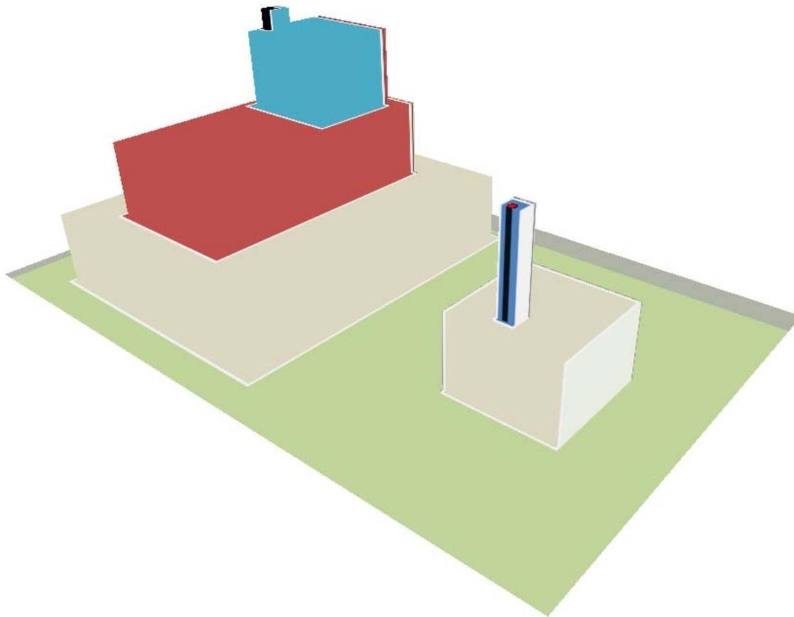
**Figure 1 Calculation grid. Source is from stack on smaller building.**
